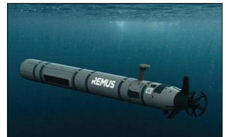
▲ Fig. 6 HII REMUS can deliver electronic warfare payloads.
